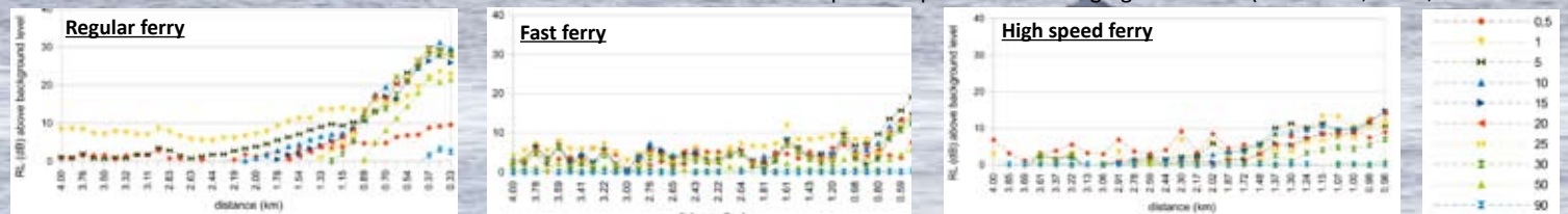
Figure 1: RL (in dB) measurements above background level for selected frequency bands (0.5-90 kHz) during approaches from a 4 km distance to CPA for the (a) fast ferry, (b) regular ferry and (c) high-speed ferry
